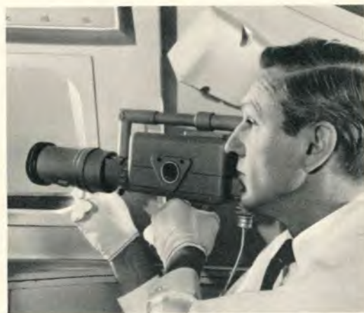
This television camera developed by Radio Corporation of America enabled live transmissions to be made from the spacecraft. The camera was fitted with a 160 degree wide-angle and a 9 degree telephoto lens. It is only 1/85 as large as those used in TV studios and has a weight of 4.5 lb.
