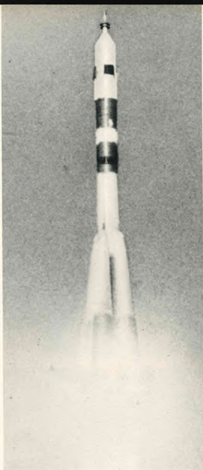
Fig. 6: Shortly after launch of the Soyuz . As with the Vostok launch, first and second stage engines are fired at the same time. — 7. Assembly of the spacecraft. The spherical living and control modules can be seen. The solar cell panels are unfolded. — 8. Astronaut Georgi T. Beregovoi in the spacecraft's roomy rest area. During his mission, he did, of course, wear a special suit.
