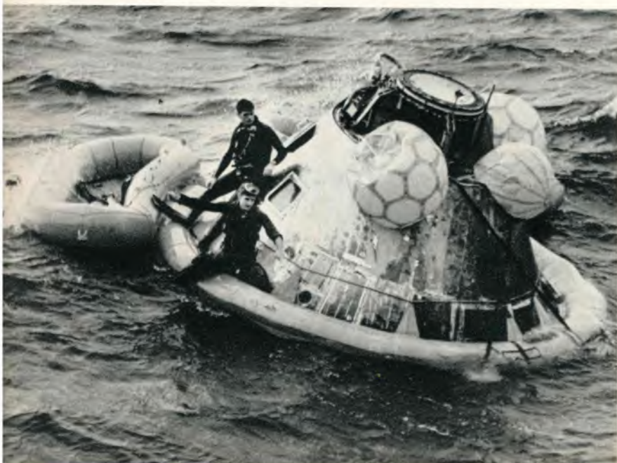
Recovery of the Apollo 8 Command Module on December 27, 1968 from the Pacific Ocean. The three balloons ensured that the Module floated the correct way up after splashdown. The ring was fitted by frogmen. A helicopter transported the three astronauts to the aircraft carrier Yorktown ; later they were flown via Hawaii to Houston, where they reported on their mission.
