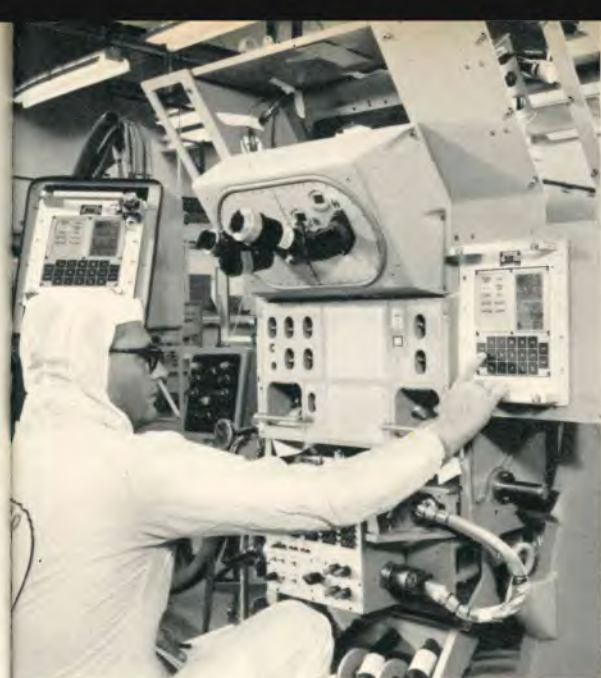
The Apollo spacecraft and the lunar module has a guidance and navigation system produced by the General Motor AC Electronics Division. The picture shows an AC technician carrying out systems tests. The main contractors for the spacecraft and the lunar module are North American Rockwell and Grumman respectively, although nearly all large firms in the American aerospace industry have participated in the Apollo programme.
