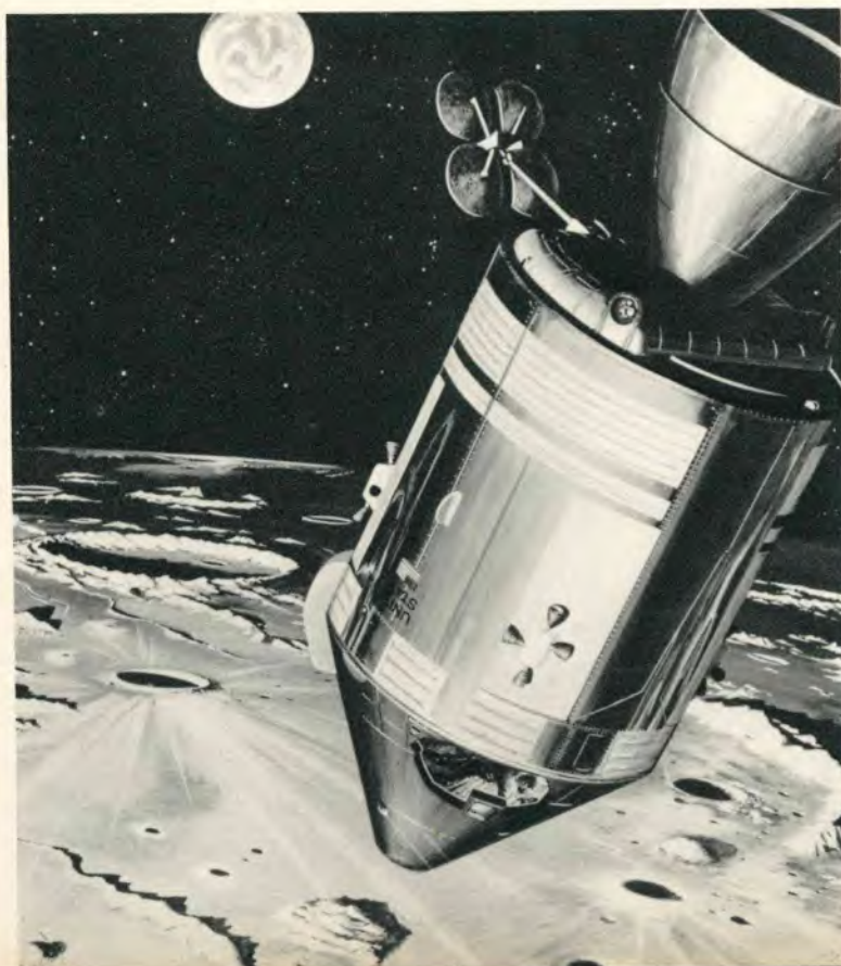
This artist's impression shows the Apollo 8 in lunar orbit. In the cutaway section of the command module, one of the astronauts can be seen observing the lunar surface. The astronauts took many photographs and films, having at their disposal two 70 mm Hasselblad still cameras with two 80 mm lenses and a 250 mm telephoto lens, and also a 16 mm Maurer ciné camera with 5, 18, 75 and 200 mm lenses, as well as black and white and colour films of various sensitivities for interior and exterior photography.
