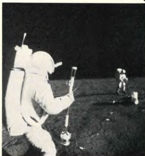
LM pilot Ed Mitchell operating the "Thumper" as part of the Apollo 14 Active Seismic Experiment (see text). In the background is Mission Commander Alan B. Shepard Jr.
