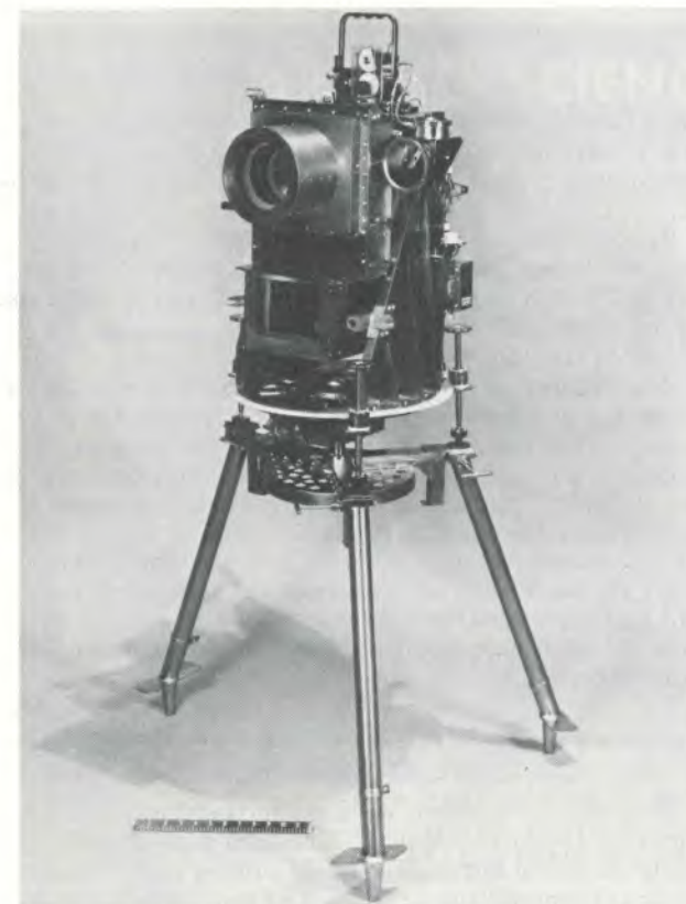
The NRL Far UV Camera/Spectrograph.
