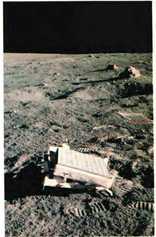
A hundred quartz mirrors make up the face of this instrument, the laser ranging retro-reflector (LR-3). It bounces laser light beams back to Earth when scientists aim them at the Moon, for distance measurements.
