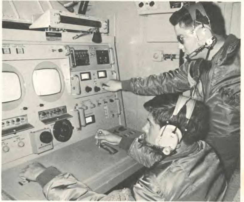
ALOTS CAMERA CONSOLE —This automatic tracking console of the Airborne Lightweight Optical Tracking System (ALOTS) mounted in an Air Force Eastern Test Range NKC-135 was used in the filming of the Apollo 11 lunar launch. After the two operators lined up and centered the picture of the Apollo vehicle, the system automatically kept it centered on the screens of the monitor.
