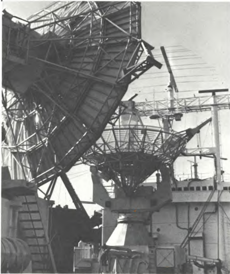
A VIEW FROM THE main deck with the Unified S-Band antenna on the right. Each of the Apollo Instrumented Ships is equipped with sophisticated tracking, telemetry, communications, data processing equipment and state-of-art navigation equipment.
