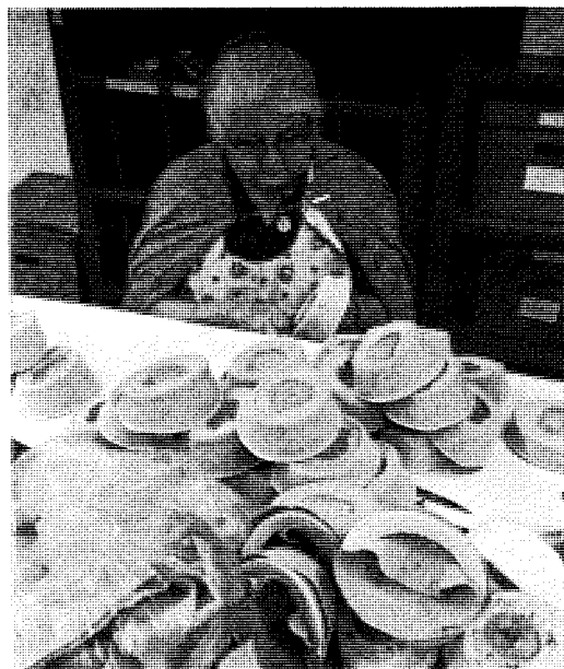
Another stage in the production of the A-7L Apollo suit: this worker is making ear cups for communications receivers/headsets.
