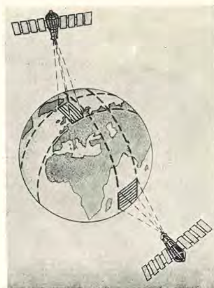
Diagram of relative location of Meteor satellite orbits The orbital inclination is 81.0 to 81.2 degrees
